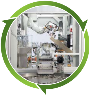
Daisy, Apple's latest innovation in material recovery, can disassemble nine different iPhone models to recover valuable materials that traditional recyclers cannot. Courtesy of Apple Inc.
