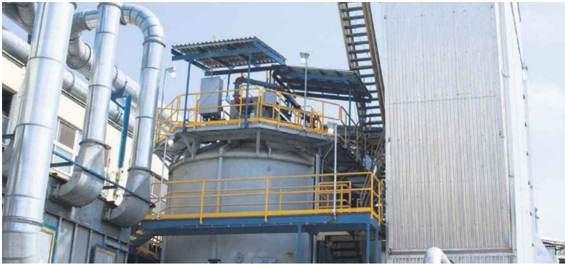
Kruger's pulp mill in New Westminster, B.C., introduced the first biomass gasification system in Canada, leading to a nearly 60 per cent reduction in CO 2 emissions. SUPPLIED
