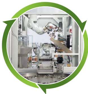
Daisy, Apple's latest innovation in material recovery, can disassemble nine different iPhone models to recover valuable materials that traditional recyclers cannot. Courtesy of Apple Inc.
